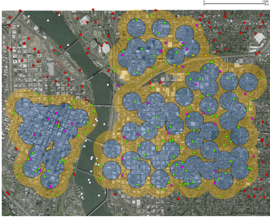
Fig. 3: Random locations and their categorization. Green (light-grey) dots were tested, purple and orange (grey) were points within the POC that were excluded because they were inaccessible, and red (dark-grey) were excluded because they were not within the POC.
