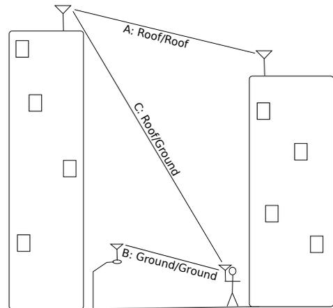
Fig. 1: Visual schematic of three urban datasets. **A**: roof to roof measurements from CU WART (Wide Area Radio Testbed), **B**: ground (light-poles) to ground (mobile node) measurements in Portland, Oregon, **C**: roof to ground and ground to roof measurements from CU WART.
