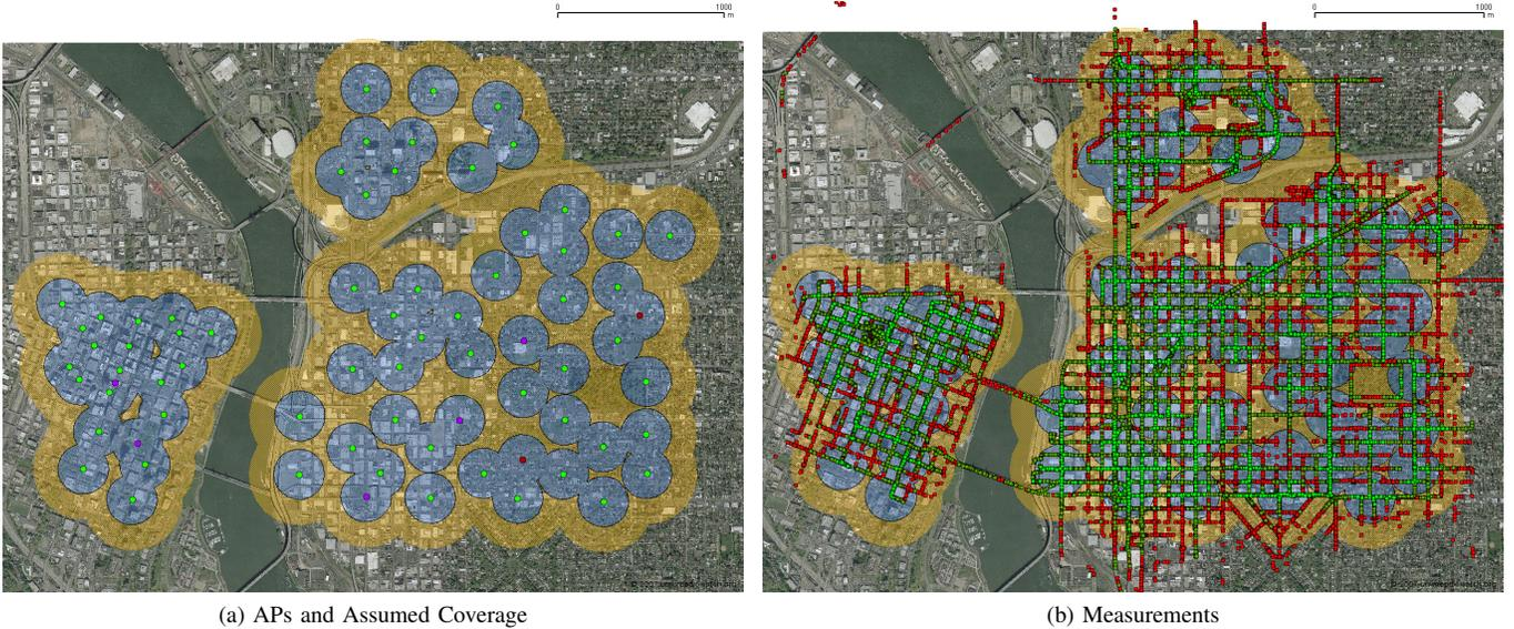
Fig. 3: Portland MetroFi network with operator-assumed coverage. Lighter dots (green) indicate stronger signal. 500 ft. and 1000 ft. radii circles are placed around each AP to show the operator assumed coverage.
