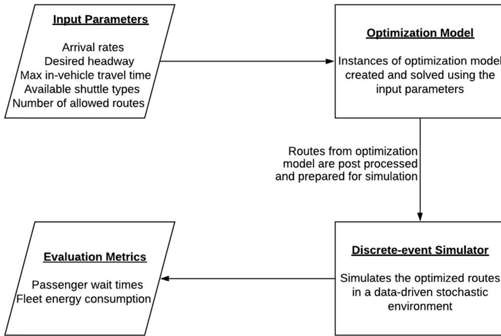
Fig. 1. Route optimization for energy efficient airport shuttle operations: process flow chart.
