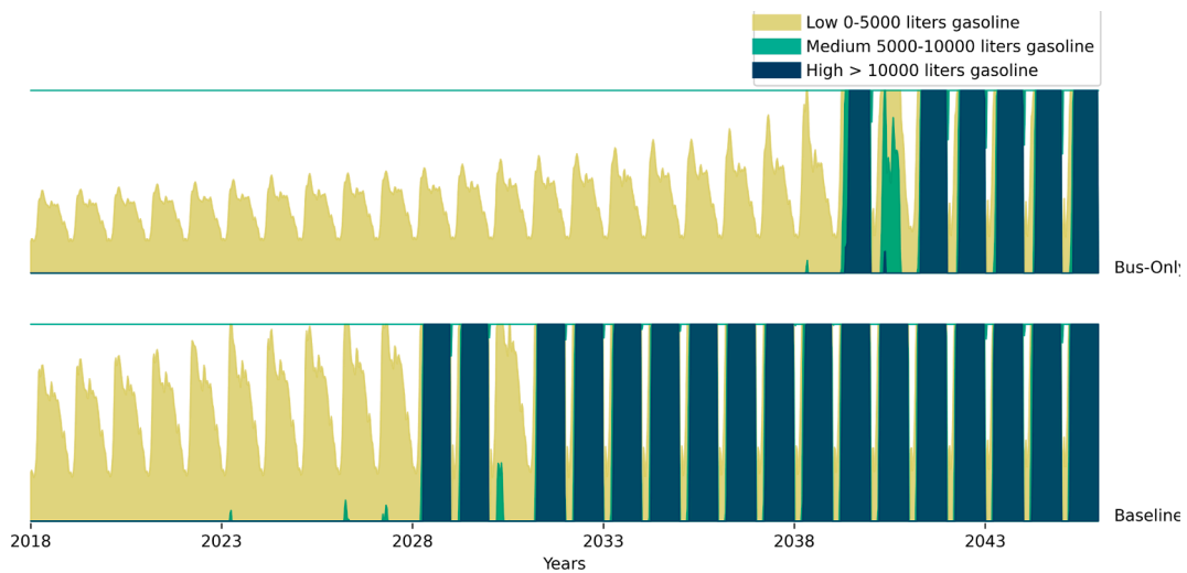
Fig. 17. Time of day fuel consumption of base case and buses-only scenario for high demand day projected to 2045.
